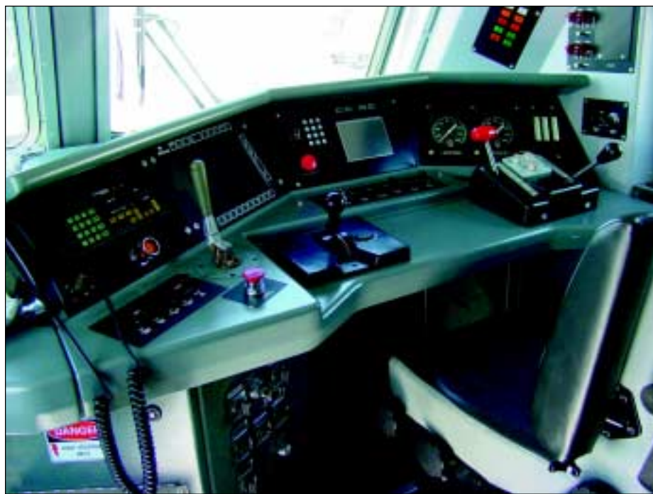
Control panel of the ALP-46.
